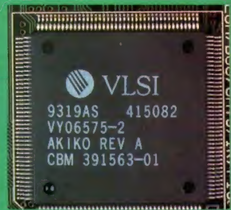
The special custom chip on the Amiga CD 32 automatically handles the conversion of pixels' colours much faster than the processor could do it.
